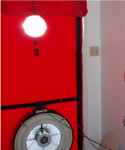
A blower door test is set up in an entryway to change the indoor pressure of your home, helping to identify leaks.
